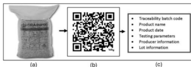
Figure 8. Product identification with QR code. (a) Coffee sample with a QR code printed on the surface; (b) an amplification of the QR code; (c) product information stored in the QR code.
